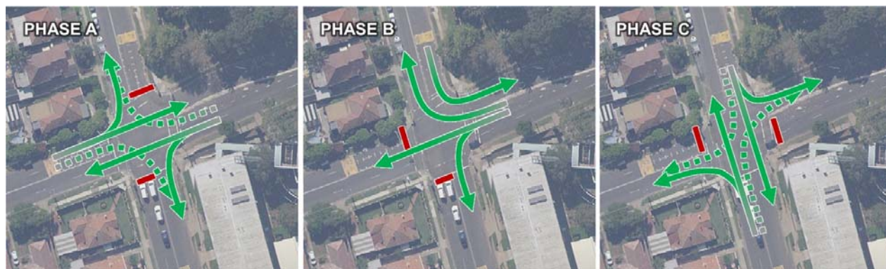
Figure 5-4: George Street / Pomeroy Street Current Phase Sequence
