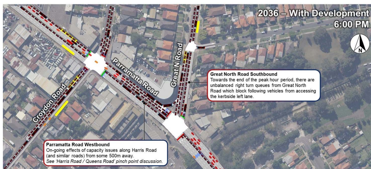
Figure 4-20: Parramatta Road / Great North Road Pinch Point
