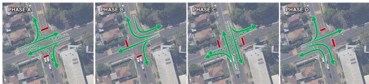
Figure 5-5: George Street / Pomeroy Street Proposed Phase Sequence
