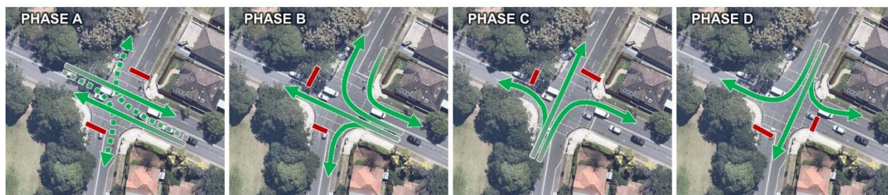
Figure 7-9: Gipps Street / Broughton Street Proposed Phase Sequence
