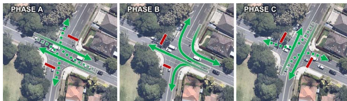
Figure 7-8: Gipps Street / Broughton Street Current Phase Sequence
